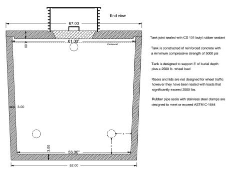
Tank is constructed of reinforced concrete with a minimum compressive strength of 5000 psi
